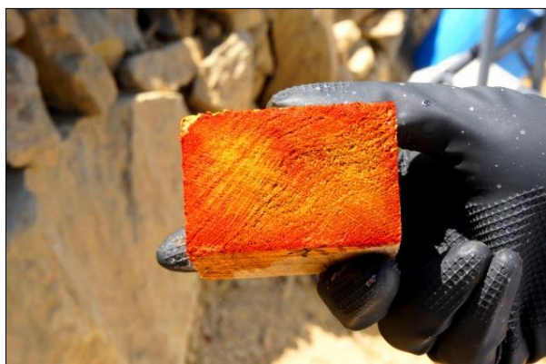
Wood section that shows a homogeneous concentration of DOT solution.
